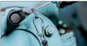
Use of ratchet. The ratchet does not have a button for switching sockets like a standard ratchet.
