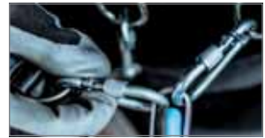
The carabiner on the lanyard has to be protected against opening using a lock ring.
