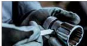
Using the socket remover (Article 1111) depress the pin in the hole while removing the socket from the square drive of the ratchet and then switch the socket or extension.
