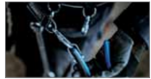
Correct attachment of the tool to the lanyard. Return the tool to the belt following the steps in reverse order.
