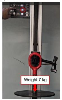
• In second step it requires to hang on the weight in the range between 15 kg and 25 kg., as indicated by value 15 on upper display an 25 on lower display. Repeat the process of setting the middle-display number to match real weight on the master arm. Then confirm this step by holding the STOP button pressed again for about 3 seconds (in our case, we hung 7 kg on the master arm and set the number 17 on the control panel as shown on picture below.
