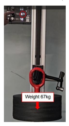
After confirming the third step the stand will automatically exit calibration mode and will be ready for use.
