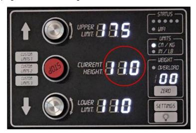
2. Hold the button on the control panel for about 1 second to enter the settings menu and press the button once again to enter calibration page, as shown on picture below.
